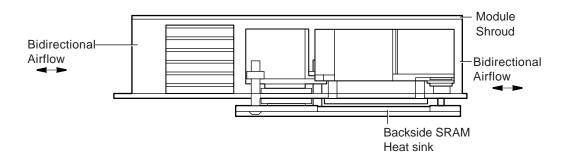
Figure 8. CPU Module Side View
